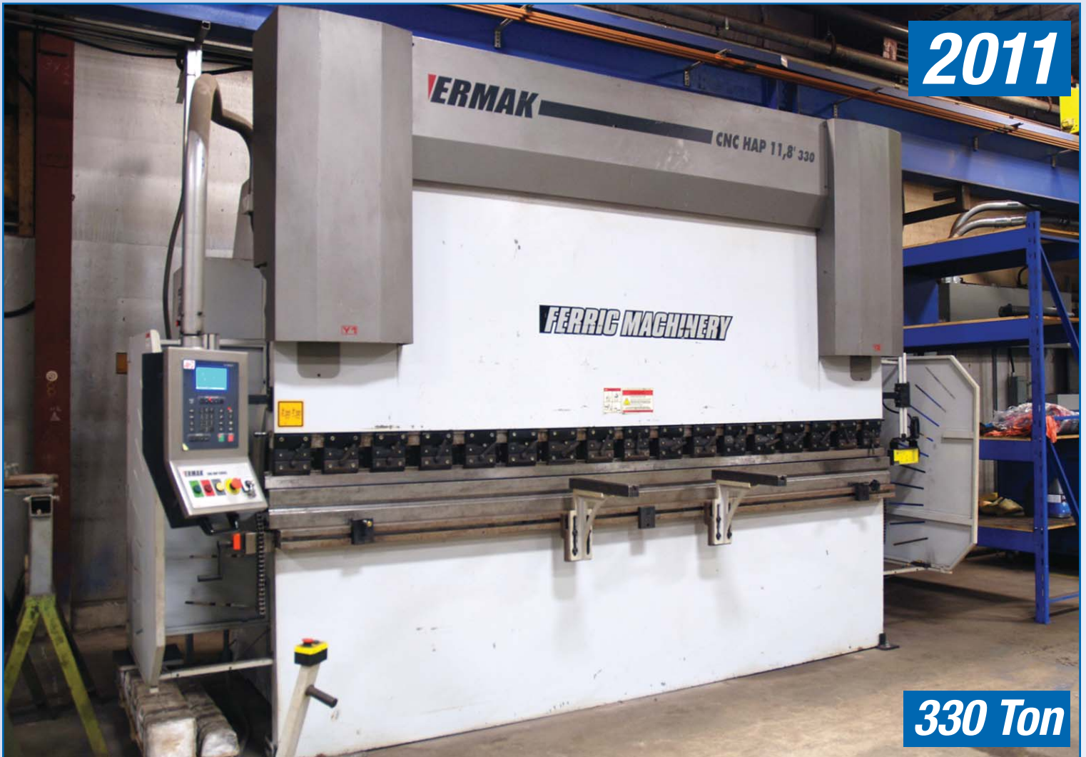
ERMAK 11'10" x 330 Ton CNC Press Brake, Model CNC Hap 11x330, 3 Axis, Cybelec DNC 60 Control, Manual Crowning, Fiessler Laser Light Curtains, 10'5" Between Frames, 16" Throat, 12' 4 Way Die (may be sold separately), 30 HP, 575V, sn 02096-PJC4KX
