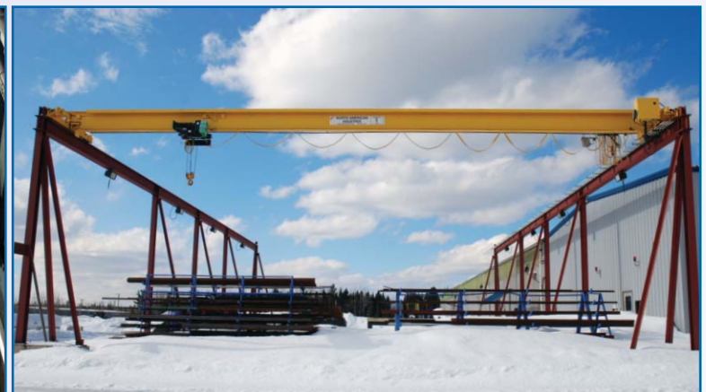
NORTH AMERICAN INDUSTRIES 5 TON 60'X90' SELF STANDING OUTDOOR CRANE
